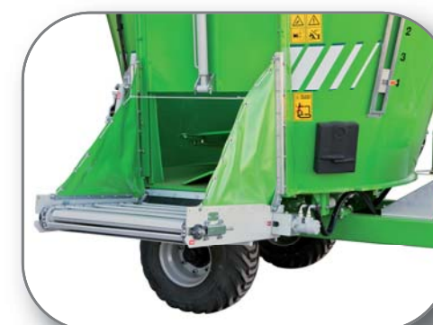
Hydraulic elevator on side door.
